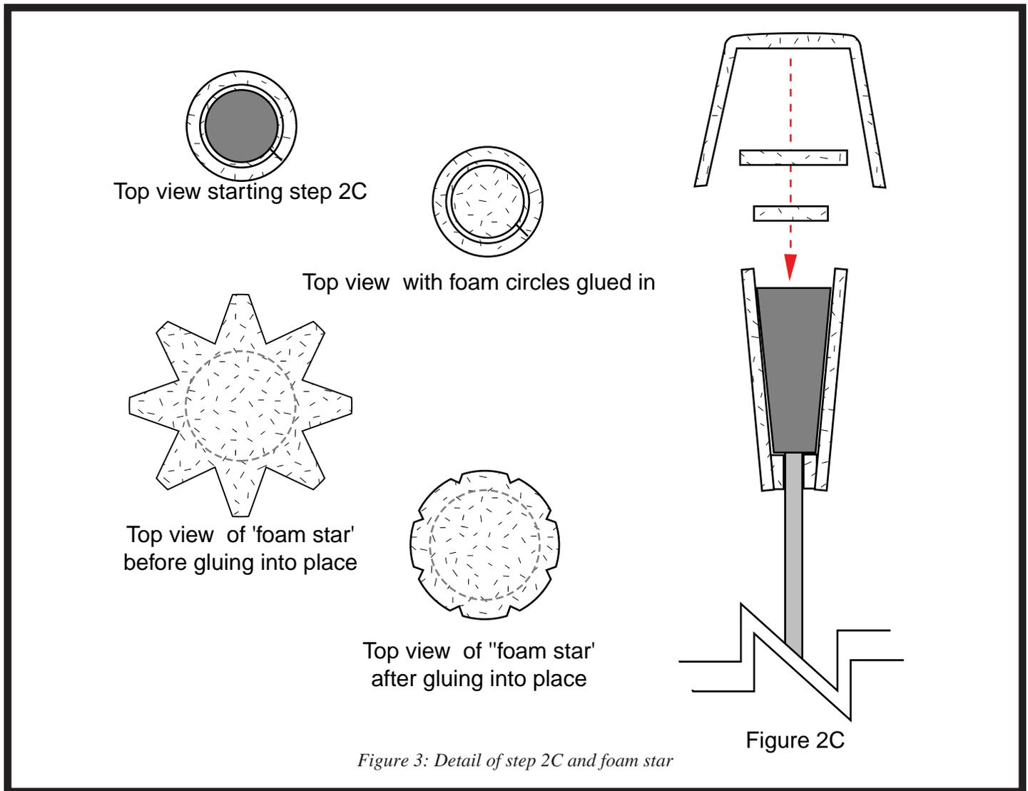
Figure 3: Detail of step 2C and foam star
