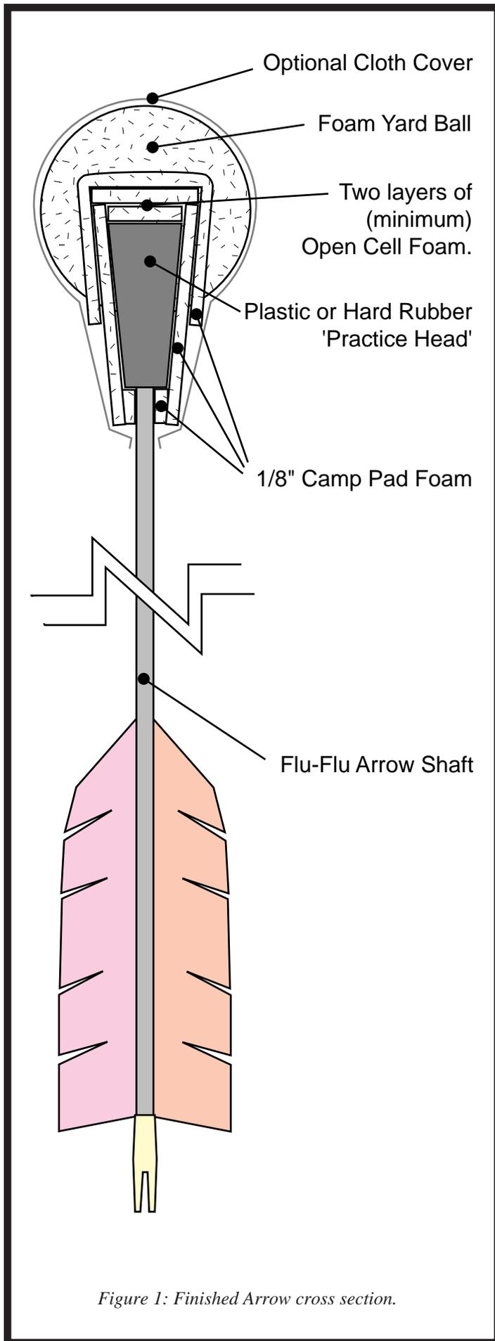
Figure 1: Finished Arrow cross section.
